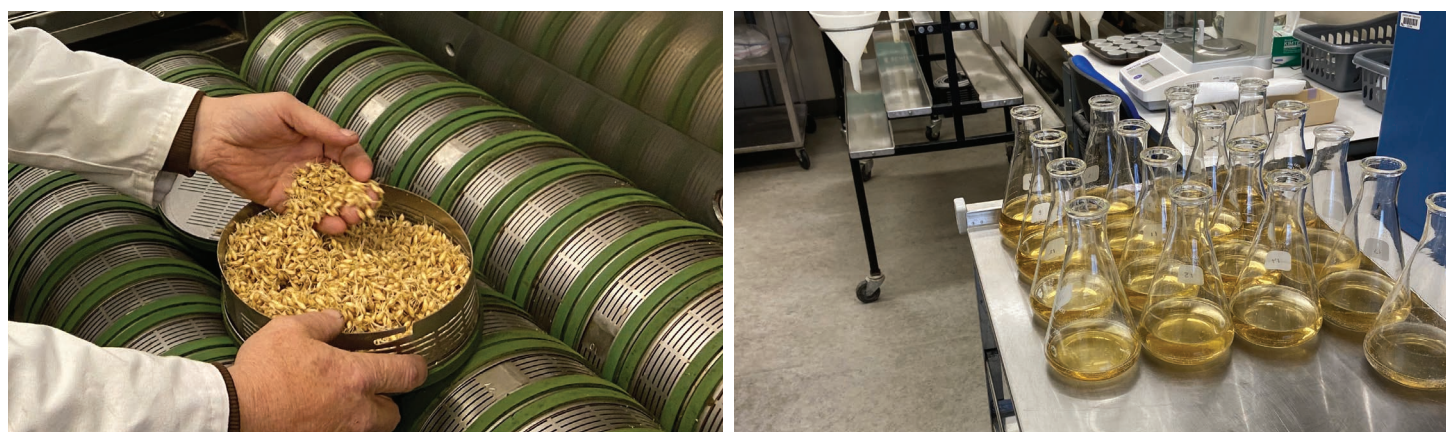
Examining barley during malting in the Phoenix Micromalting System (left) and wort samples collected after the mashing of malt (right) at the malting lab of the Grain Research Laboratory.
