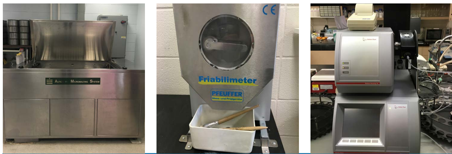
Phoenix Micromalting System (left), friabilimeter (middle), and densitometer (right) at the malting and malt analysis labs of the Grain Research Laboratory.
